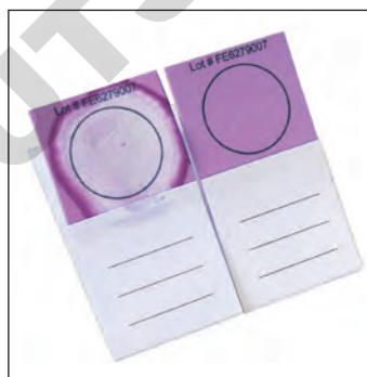
Indicating FTA Elute Micro Card with buccal sample (left) and no sample (right).
