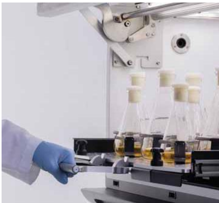
Conveniently reach all areas of the shaker platform and chamber using the slide-out tray
