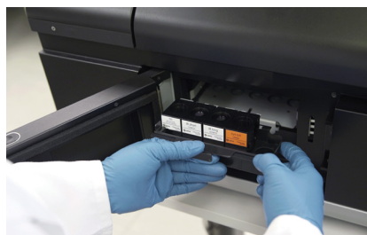
Fig 2. Users can easily exchange the filters in Amersham Typhoon 5, RGB, NIR Plus, and NIR models. If a new filter is inserted or a filter is changed, the instrument automatically recognizes the filter and updates the control software.
