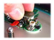
**NOTE:** The upper measurement chamber plate is still connected to the lower housing by a ribbon cable. Do not loosen or remove the ribbon!
