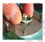
**Important:** Make sure you mount back the cover correctly. Special care has to be taken for the 4 screws fixing the cover to the cover plate. Screw them tightly. If cover is not closed properly, measurement problems can occur
