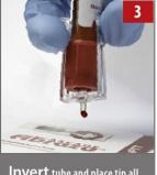
**Invert** tube and place tip all the way into sample well until it reaches the bottom.
