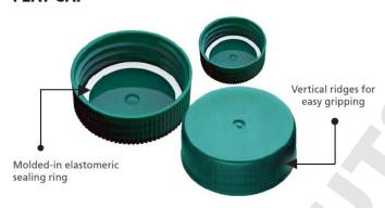
**FLAT CAP**: offers unsurpassed sealing. Both 15mL and 50mL flat caps include an integral molded-in elastomeric sealing ring that eliminates leaking. With their smooth surface, flat style caps can be easily labeled and are designed to produce an evaporation proof seal with a ¾ turn for one-handed operation plus a final ¼ turn to seal them liquid tight.
