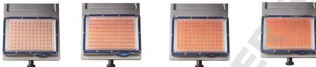
Figure 4: Filling a 384 well plate in four steps with a 384 well adapter positioned by a wheel
