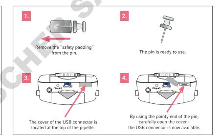
4. Connect and update the pipette with the Pipette Manager
