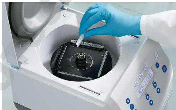
Centrifuge 5420 offers two rotor options: A 24-place standard rotor for up to 24 × 1.5 or 2.0 mL tubes and a PCR-tube rotor for 4 × PCR strip or 32 × PCR tubes (0.2 mL).
