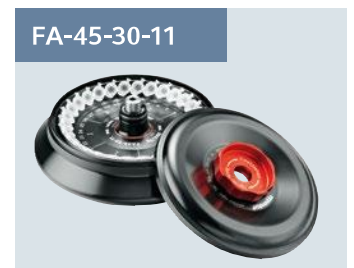
FA-45-30-11 30 × 1.5/2 mL micro tube rotor with aerosol-tight lid for safe centrifugation of hazardous samples. Max. speed 20,800 × g (14,000 rpm).
