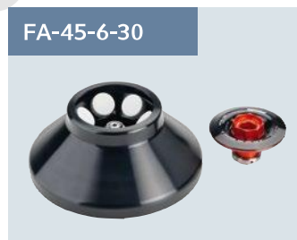
FA-45-6-30 6 x 50 mL conical tube rotor with aerosol-tight QuickLock lid for tubes from 5–50 mL. Max. speed 16,639 x g (11,000 rpm).
