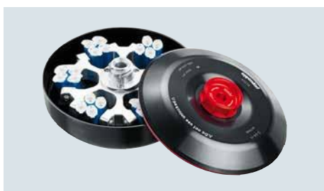
Swing-bucket rotor for 24 × 1.5/2.0 mL tubes spins up to 16,050 × g /12,700 rpm. Swing-bucket design is ideal for phase separation (S-24-11-AT*; Order no. 5409 715.003).
