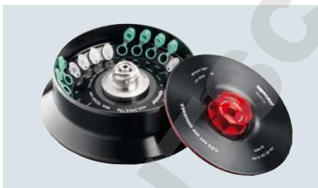
Eppendorf Kit rotor for 24 × spin columns and 1.5/2.0 mL tubes. Designed with an extra high rim to support open tube lids during centrifugation. Spins at max. 19,100 × g /13,200 rpm (FA-45-24-11-Kit*; Order no. 5409 704.001).
