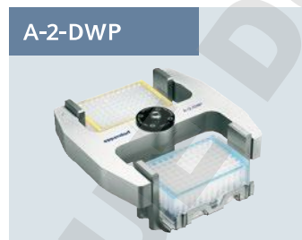
A-2-DWP 2-place deepwell plate rotor for plates up to 89 mm loading height. Max. speed 2,250 × g (3,750 rpm).
