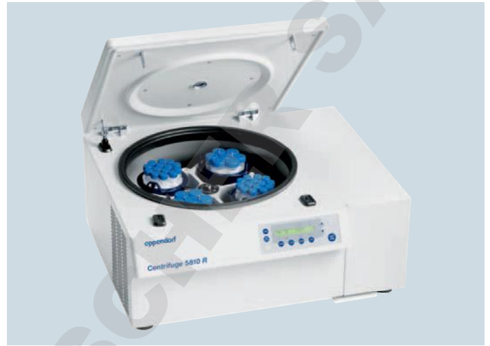
Centrifuge 5810 R rotor S-4-104 (4 x 750 mL)
