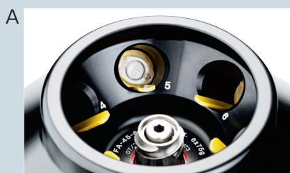
Figure 4: a) Rotor FA-45-6-30 (Centrifuges 5804/5804 R and 5810/5810 R) for 6 tubes with adapter for 50 mL bore. b) Adapter for 50 mL bore
