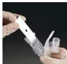
Place new filter onto microscope slide.
