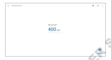
Set up the required measurement parameters. Insert the cuvette containing the blank solution into turret position 0 followed by the cuvettes containing the samples into turret positions 1 to 7 and close the instrument lid.
