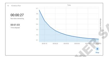
Once the measurement time is complete the full kinetics run will be shown on the screen. To run the kinetics experiment again using the same method parameters touch RUN AGAIN. Subsequent samples can be measured in the same way. If the wavelength is adjusted between sample measurements then the instrument must be calibrated again before more samples can be measured.
