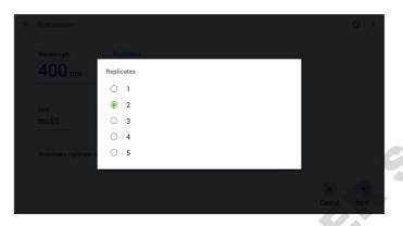
If 2 or more replicates are selected, Automatic replicate measurement becomes active. Automatic replicates will read the same sample for the selected number of replicates. If individual sample replicates are being used, do not select the automatic replicates option.
