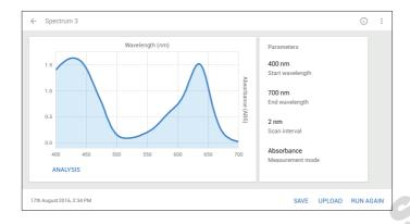
Once the spectrum scan is completed it is possible to analyse the spectrum scan. Post measurement tools include peaks and valleys and area under the curve. To analyse the data touch ANALYSIS.
