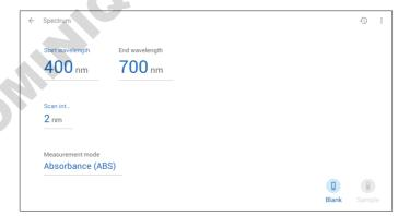
The start and end wavelengths must be different. If the same value is entered an error message will be displayed.
