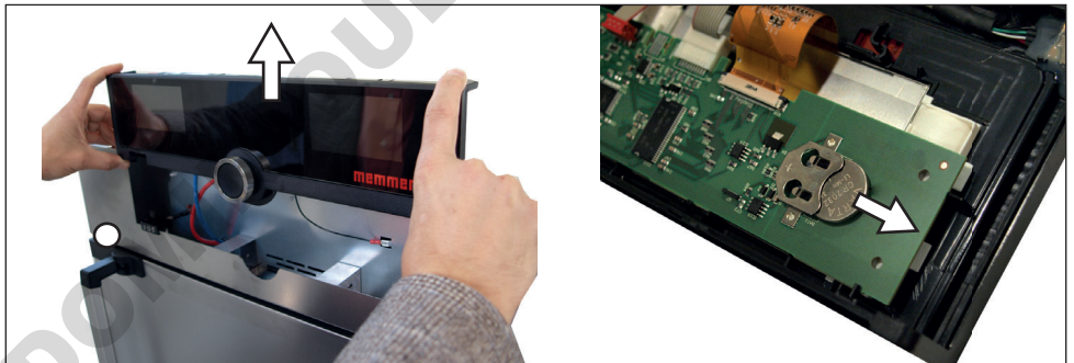
Fig. 34 Removing the lithium battery
