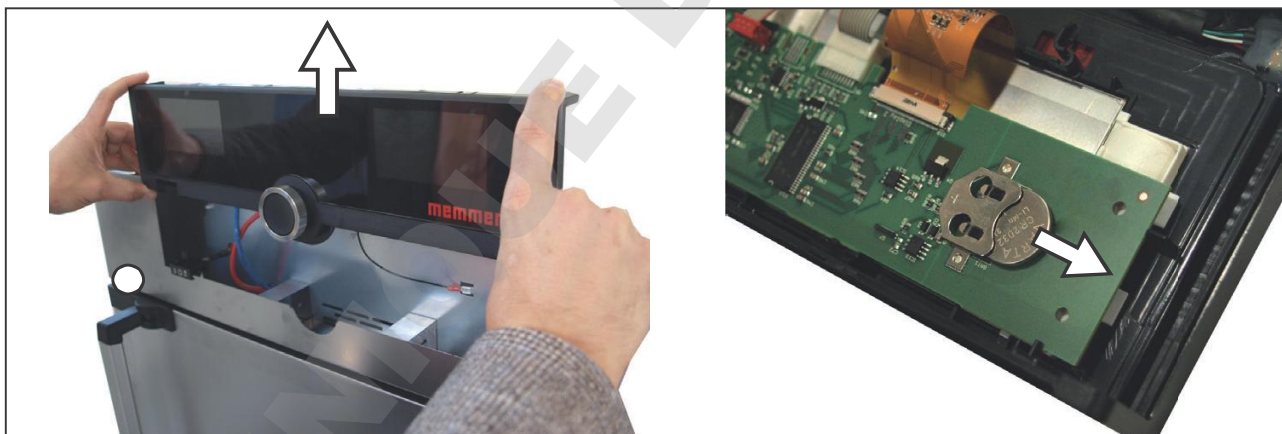
Fig. 25 Removing the lithium battery
