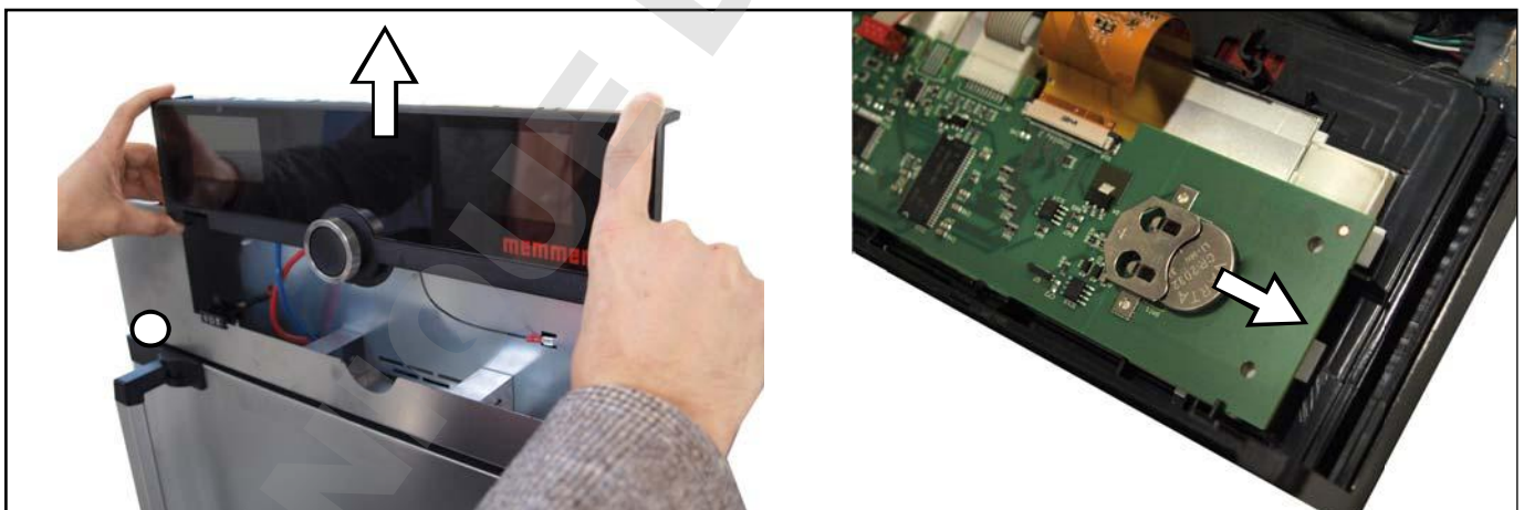
Fig. 25 Removing the lithium battery
