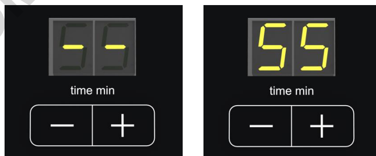
Fig. 13: Time setting for continuous operation (left) or with a process time (right)
