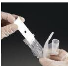
Place new filter onto microscope slide.
