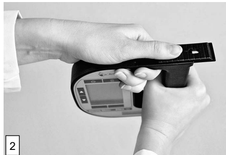
Fig. 11: Removing the pump lock screw (1) and the pump lock (2)
