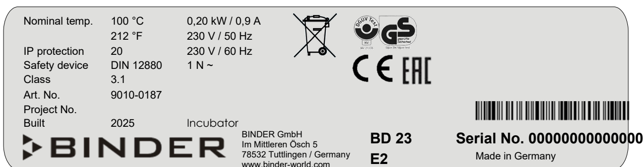
Figure 2: Plaque signalétique (exemple BD 23 standard)
