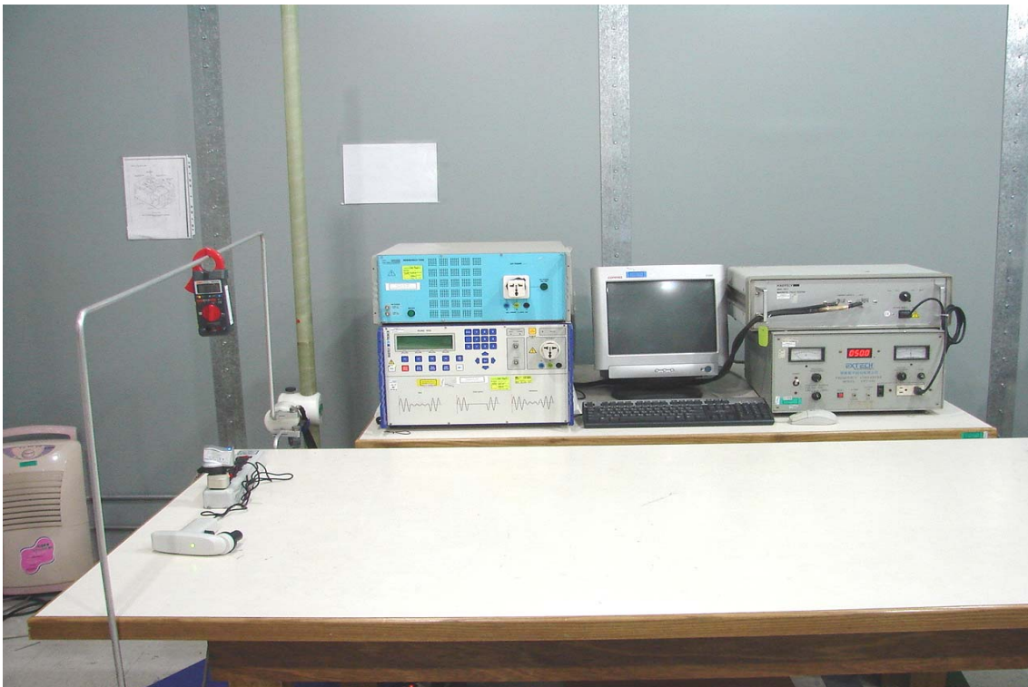
POWER FREQUENCY MAGNETIC FIELD IMMUNITY TEST
