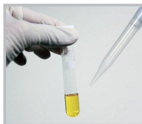
1. Pipet 2.00 ml sample into a COD vial
