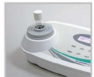
3. Detect the reagent vial to get COD value
