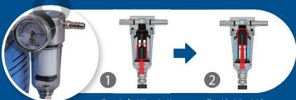
Once the liquid is sucked into the moisture trap accidentally, the buoy of Prote™ overflow protection will float up. Then block the air inlet to prevent the liquid from flowing into the pump.
