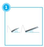
CELLstage guarantees an exact filling angle of 30° for CD4-CD24 (878072) and 20° for CD40 (878073).
