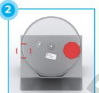
Position CELL disc™ on the filling accessory with the screw cap either at 105° for right-handed users or 255° for left-handed users (indicated by ( )).
