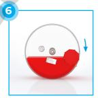
For liquid equilibration, take CELLdisc™ out of the CELLstage, lay it down horizontally and turn it to assure that the medium and all layers are in contact through the central filling channel.
