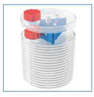
6 The other CELLdisc™ can now be positioned on top of the CELL-evator™. Ventilation of the lower CELLdisc™ is assured by the notches on the segments whereas planarity of the upper CELLdisc™ is assured by the elevations on the segments.
