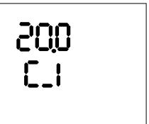
b) Pressing "Temp" or "Temp" to set the first calibration temperature point as 40°C.
