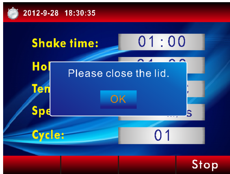
Figure 4.28 The open lid alarm interface
