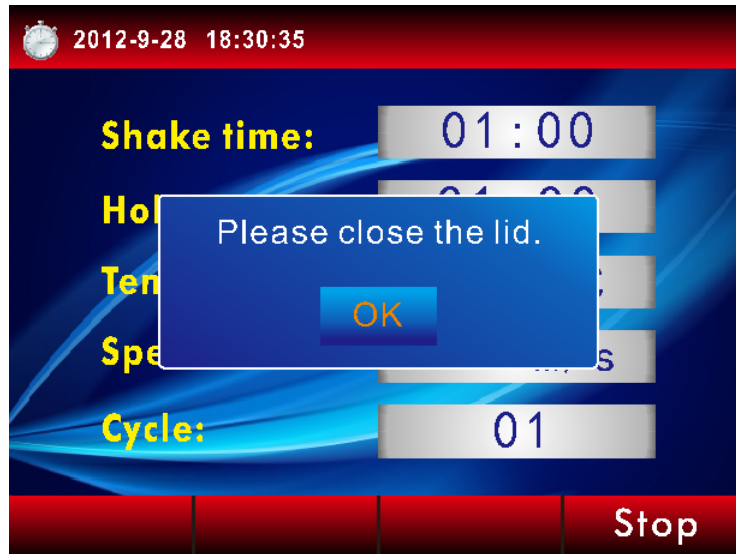
Figure 4.30 The open lid alarm interface
