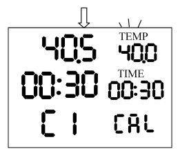
When the calibration of  $40^{\circ}$ C is done, press "  $\frac{\text{start}}{\text{Stop}}$ " to exit; at this time the calibration of  $40^{\circ}$ C is ineffective.
