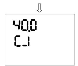
c) Perform the same operation again to set up the second calibration temperature such as  $100^{\circ}$ C;
