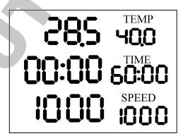
c) Press " speed" or " speed" to set up for the speed. The number will increase or reduce at a rate of 50rpm, release the button when the number reaches exact value, and it will be automatically saved in 3 seconds.
