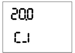
**b**) Press the temperature set up button "  $\begin{tabular}{l} \end{tabular}$  or "  $\begin{tabular}{l} \end{tabular}$  " to set up the first calibration temperature such as 40%;
