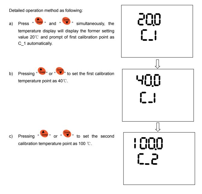
Note: It is recommended to set calibration points from low temperature to high temperature.
