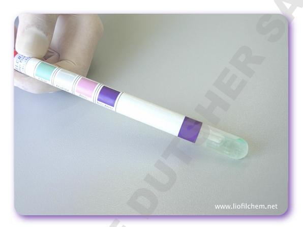
Swab for detecting protein, fat and sugar residues for the hygiene control of surfaces
