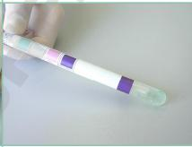
Insert the swab into the tube and push the tube in order to lower the swab tip close to the disc.
