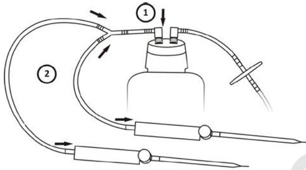
If more than one handle is used – for the multi-user systems AA 02 and AA 04 as well as for the two-user system AA 24 – the unused handles must always be closed since otherwise no vacuum can be generated in the bottle.
