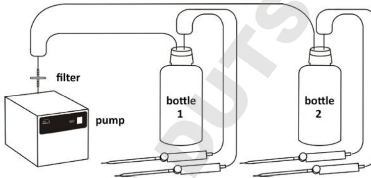
In both cases it is required that the Y-manifold AY 01 of HLC by DITABIS is used for connecting the bottles since this ensures a straight-line connection to the fast-lock caps of the bottles (see description "Assembly AA24 for 2 Workplaces").
