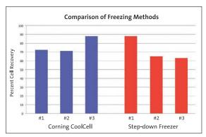
Graph comparing percent of cell recovery after freezing with the Corning CoolCell freezing device (blue) versus freezing using a programmable step-down freezer (red) in 3 different samples at high cell concentration. There was no significant difference between the two freezing methods. (Data generated by UCSF Diabetes Center)
