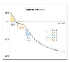
A temperature probe was placed into a 2.0 mL cryogenic vial containing 1.0 mL of water, and the tube was inserted into a room temperature Corning CoolCell. The CoolCell was placed into a -80°C freezer, and the temperature rate and profile was recorded over a 3-hour period. The test was repeated 5 consecutive times. Corning CoolCell generated identical fusion time and cooling profiles over five consecutive freeze cycles.
