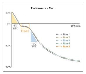
A temperature probe was placed into a 2.0 mL cryogenic vial containing 1.0 mL of water, and the tube was inserted into a room temperature Corning CoolCell. The CoolCell was placed into a -80°C freezer, and the temperature rate and profile was recorded over a 3-hour period. The test was repeated 5 consecutive times. Corning CoolCell generated identical fusion time and cooling profiles over five consecutive freeze cycles.
