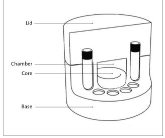
Corning CoolCell LX uses a combination of uniform-density cross-linked polyethylene foam, a solid state core, and radial vial symmetry to create freezing profiles that are consistent and reproducible. The low heat content also ensures that CoolCell LX containers will rapidly return to room temperature when removed from the freezer.
