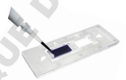
4. Insert the EVE™ Cell counting slide, sample side (side A) first into the slide port on the instrument, you will hear a soft click, if the slide is pushed in correctly. Each slide is counted separately.
