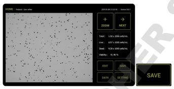
2-1) SAVE button on the main screen. In case of save to USB immediately after cell counting.
