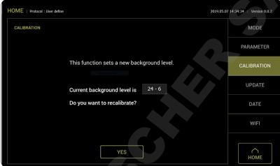
2. Check the current background level and press YES button to recalibrate.
