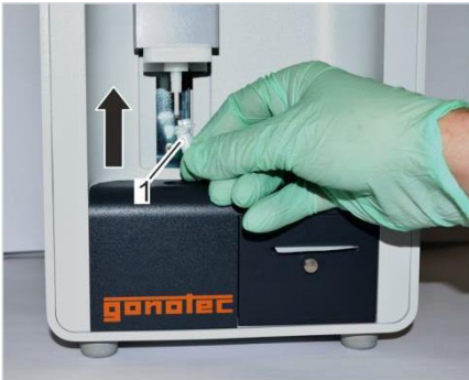
Fig. 118: Position measuring vessel
