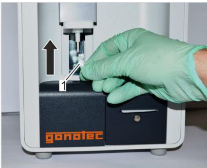
Fig. 50: Position measuring vessel
