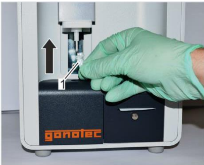
Fig. 18: Position measuring vessel
