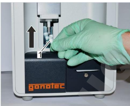
Fig. 85: Position measuring vessel
