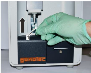
Fig. 136: Position measuring vessel
