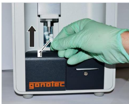
Fig. 73: Position measuring vessel
