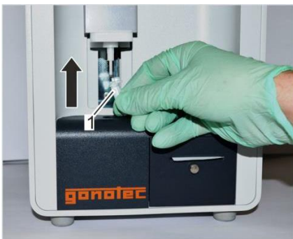
Fig. 38: Position measuring vessel
