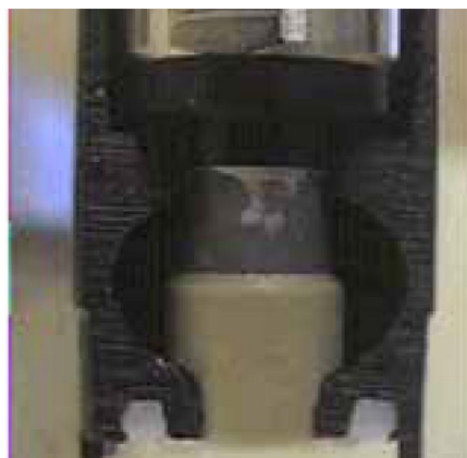
Fig. 3 Cross-section through a galvanic dissolved oxygen sensor
