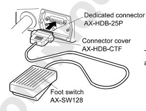
The external input connector (AX-HDB-25P/CTF) and the foot switch (AX-SW128) are sold separately.
