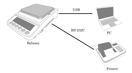
$\Box$  When connecting the balance to a PC and to the external display unit, connect the balance to the PC with a USB cable and connect the balance to the printer with an RS-232C cable.
