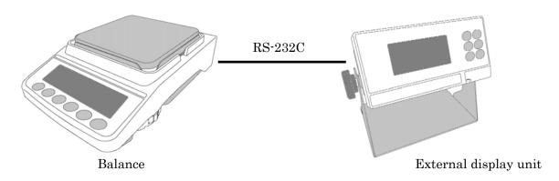
□ When connecting the balance to an external display unit and a printer, connect the balance with the external display unit (external controller AD-8922A only) with a RS-232C cable and connect the external display unit and the printer with a RS-232C cable.
