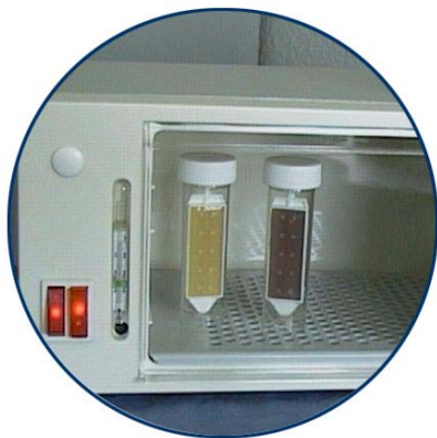
Fig. 1: Incubator for 24h incubation, and optical evaluation of a paddle tester.
