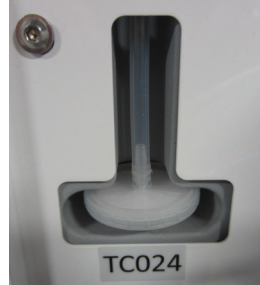
Figure 12. Tank vent filter.
