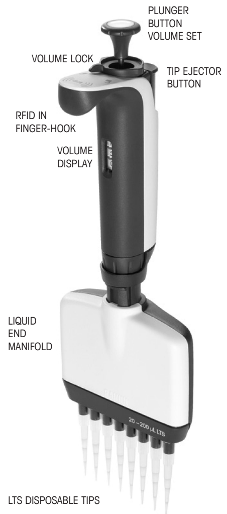
Figure 11: Pipet-Lite XLS+ Multichannel Pipette
