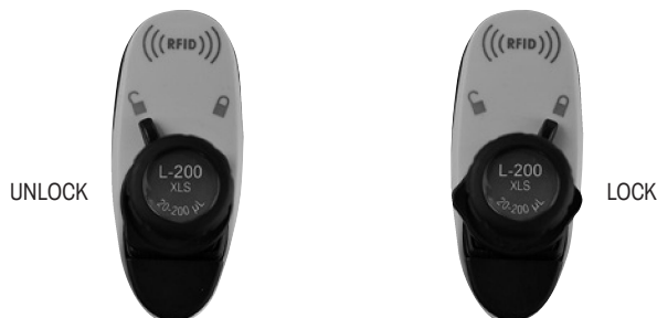
Figure 2: Volume Lock Control
