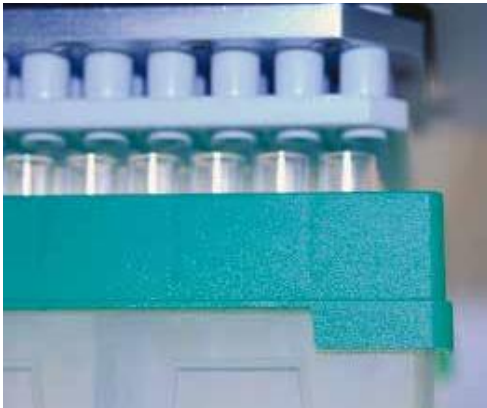
Figure A3: Non-aligned nozzles (exaggerated view)
