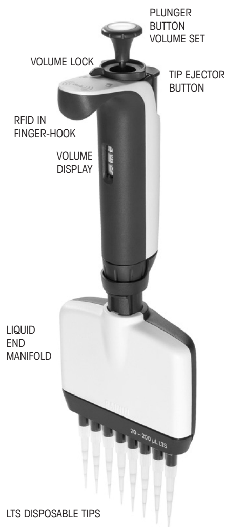
Figure 11: Pipet-Lite XLS+ Multichannel Pipette
